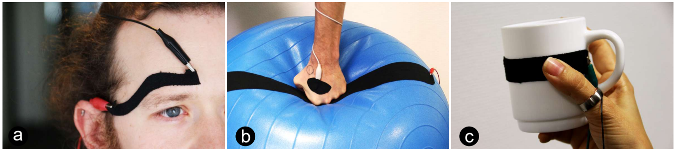
Figure 1: Polymerized tape for prototyping input devices. Here tape is used to create functional analog input on (a) the face (b) a soft, elastic object and (c) a rigid object. The elasticity and stickiness of the tape enables robust and effortless deployment, while the functional properties created by polymerization with pyrrole enable high resolution sensing.
