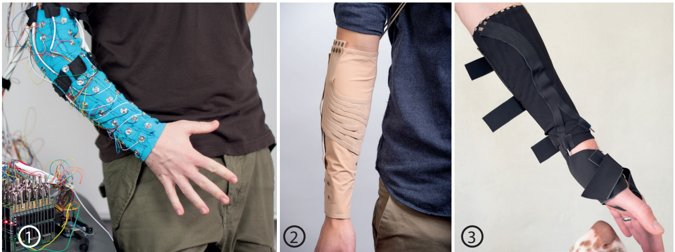
Figure 1: Wearable Electrode Sleeves. (1) The Calibration Sleeve; (2) the Manufacturing Sleeve; and (3) the Typing Sleeve.
