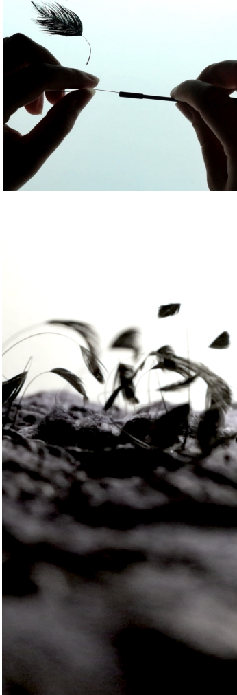
Figure 4: Top: connecting feather stems to wires with wrapping tools. Bottom: Final textile, augmented with conductive feathers.
