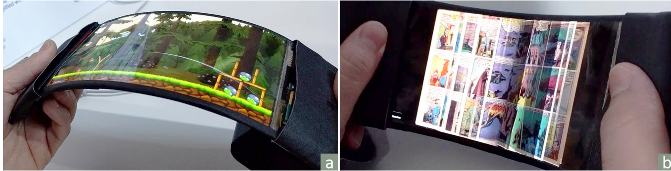
Figure 4: ReFlex is a flexible smartphone which can sense its own deformation and provide high-resolution haptic feedback [17]. Two types of mapping between input method and feedback type lead to material experiences: (a) Vibrotactile impulses are provided to the user relative to the change in strain of the device. This changes the experienced material of the device, here, providing an additional experience of elasticity. (b) Impulses are presented at a constant rate, relative to how strongly the device is bent. As they are synchronous with the pages flipping, they are experienced as a material property of the virtual book.
