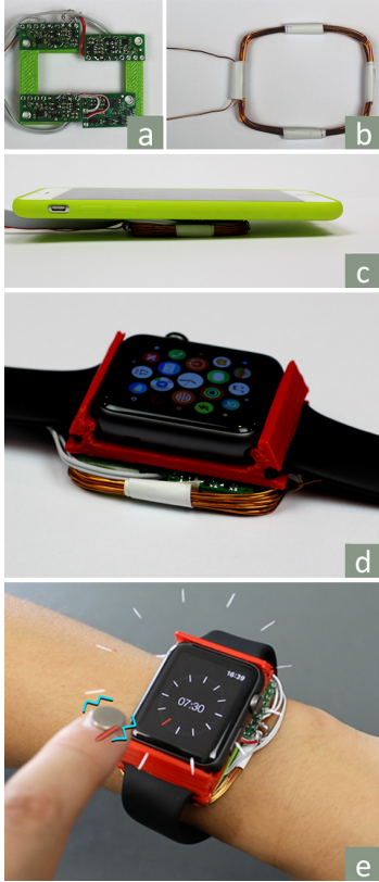
Figure 3: Magnetips consists of (a) a magnetometer array to track a magnet on the fingernail, and (b) a coil to provide haptic feedback to it. These can be used simultaneously and integrated with mobile devices (c,d) to enable interactions in the space around the watch (e) [9]. I also used the Magnetips system for providing vibrotactile feedback to an Implanted magnet [19].
