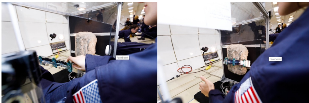
Fig. 9 Preparing to manually launch sample (left). Successful grapple moments after manual launch (right).
