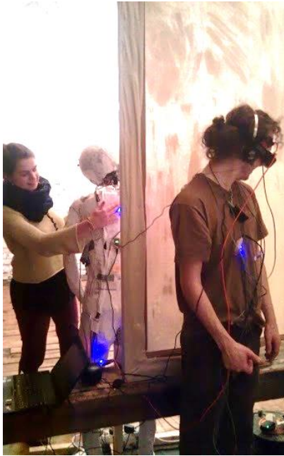
Figure 2 – A local user (left) touches the back of the robot. The remote user (right) feels a vibration at the corresponding location of his back. He sees the local user as if she were standing next to him.
